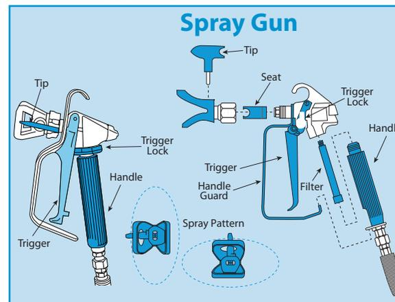
Ensure the tip is suitable for the material you wish to spray and the guns filter is the correct grade.(see table). If in doubt, contact your local HSS Hire for advice.
