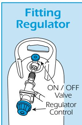
Screw the gas regulator onto the propane cylinder's valve, turning it anti-clockwise to tighten (it has a reverse thread) and tighten up with the spanner provided, then open the cylinder valve and check for leaks.
