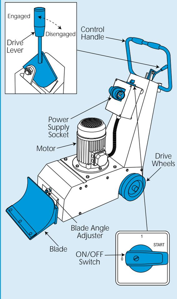
The angle of the blade can be adjusted to suit the application. To adjust, loosen the lock nut, turn the adjuster nut as required then tighten the lock nut.
