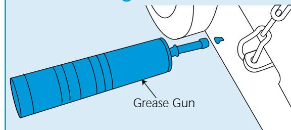
After using either model to remove 500 square metres, (long term hire only) use the grease gun provided to lubricate the blade rams.
