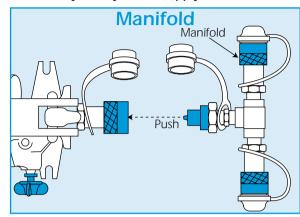
If connecting more than one hydraulic cylinder to the pump, connect a two or four way manifold.
