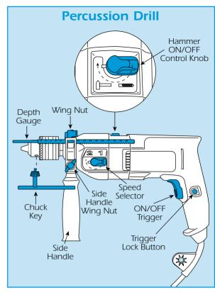
If the depth stop is to be used, this may be set either by releasing the wing nut holding it in place or by twisting the forward handgrip to loosen/tighten the depth rod's quide.
