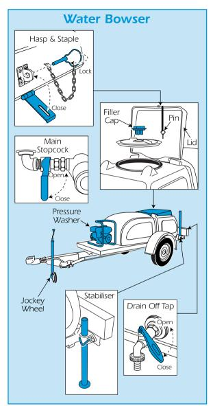
Fill the bowser until the water is no more than 300mm from the top, then turn off the supply and close and lock the filler cap.
