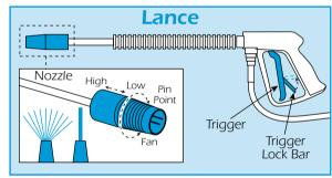
The spray pressure can be adjusted at the spray lance. For low pressure slide the nozzle forward and for high pressure slide the nozzle back.
