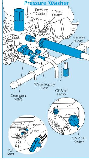
**Check the engine oil and fuel levels,** (see EQUIPMENT CARE').
