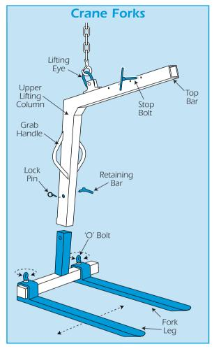
The Crane Forks are designed to lift pallet loads no greater than 1,100mm deep x 2,000mm wide x 1,650mm high. Do not exceed these dimensions.
