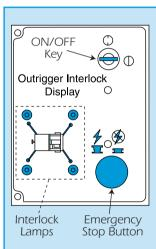
With the key inserted and turned to the ON position, the 4 interlock lamps must be illuminated before the unit will work. If any are not illuminated check the respective outrigger is correctly deployed.
