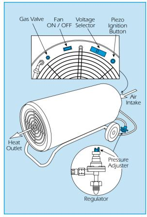
**Finally, adjust the gas regulator to produce the heat output required.** Clockwise to increase, anticlockwise to reduce.
