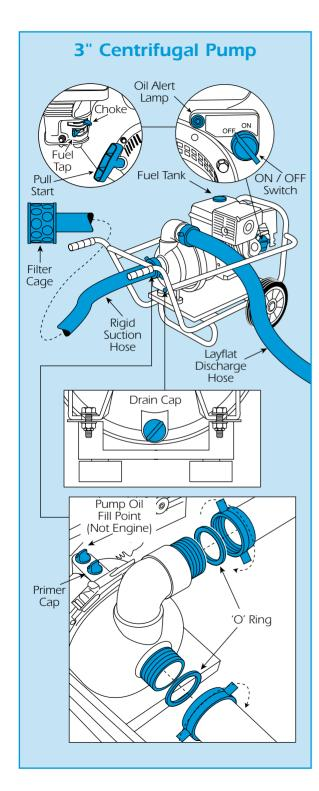
When the water level has reduced to the depth required, switch the engine OFF, lift the suction hose out of the liquid and wash off any dirt or debris.
