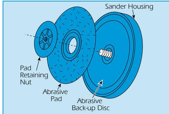
To fit a new abrasive pad (100 grit only), grasp the abrasive pad and the sander housing to prevent pad rotation.
