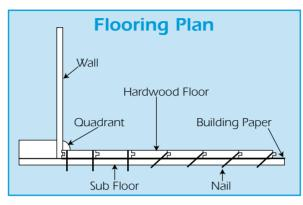
All but the last eight boards can now be fixed in place using the nailer. The last few boards must be face-nailed in the same way as the first two.
