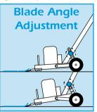
Adjust the blade angle by loosening the height adjuster knobs on the rear wheel assembly and raising or lowering the wheels.
