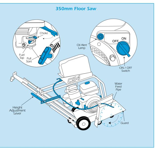
**Keep the engine upright at all times**. If it should get tipped over, mop up oil and fuel spillage's and contact your local HSS Hire Shop for advice.
