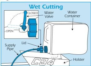
If using a wet cut wheel, you will need a good supply of fresh clean water. Turn the water valve to the closed position, unscrew the lid from the water container and fill it with fresh clean water. Refit the lid and place the container onto its holster, ensuring there are no kinks in the supply pipe.
