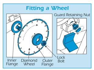
Remove the lock bolt (left hand thread) with the spanner provided, followed by the outer flange and check the condition of both inner and outer flanges. If either is damaged, return the unit to your local HSS Hire Shop.
