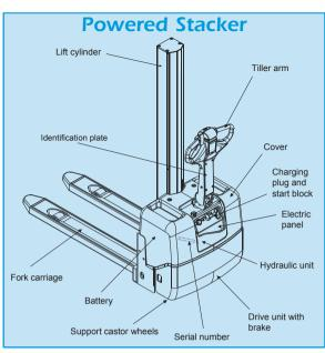
Never leave a load unattended or raised. When not in use, park the Powered Stacker on level ground where the forks will not cause a trip hazard. Ensure the work area is well lit. When moving loads keep to a sensible pace. If you go too fast, or if you try to wheel a heavy load down a slope, it could run away with you. Check the condition of the equipment before use. If it shows signs of damage or excessive wear, return it to your local HSS Depot.
