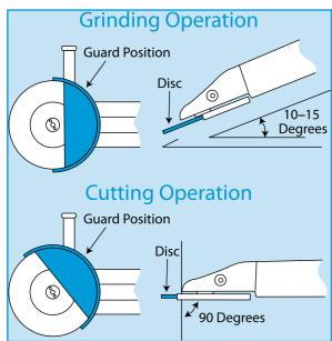
If grinding, work the tool back and forth across the surface, holding the disc at an angle of 10 to 15 degrees - a new disc may only require a single pass.
