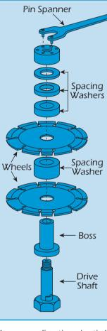
Before plugging in and switching ON, set the required chase width.
