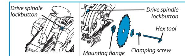
Turn the saw blade clamping screw with the hex socket wrench until the locking pin engages fully.
