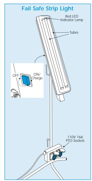
The backup supply will power the unit for a maximum of 3 hours. Note that the backup only powers one of the two tubes.
