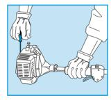
Pump the purge bulb until fuel is visible in the 'clear' fuel return tube.
