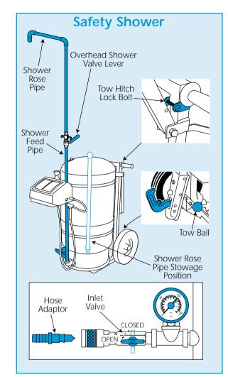
If towing the unit, unhook from any towing vehicle and stand the unit upright. Stand the safety shower on a firm, level surface strong enough to bear its weight. DO NOT use on slopes, soft ground or where there is a risk of subsidence.
