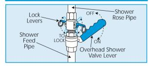
To operate the overhead shower, stand under the shower rose and move the green valve lever down. When finished, simply raise the valve lever to stop the flow of water.
