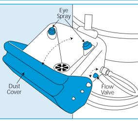
To operate the eye bath, pull the dust cover back this will automatically activate the water flow. To increase the flow rate, turn the flow valve anticlockwise, to decrease, turn the flow valve clockwise.
