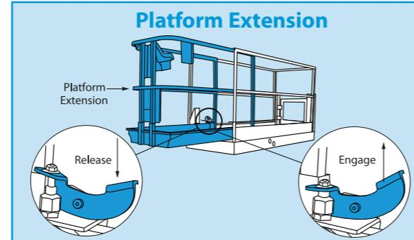
awkward areas. To deploy the extension, depress the platform extension release pedal with your foot and push the platform extension with the guardrail.
