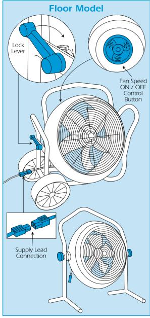
Now choose the direction of the air-flow in both the horizontal and vertical plane by loosening the appropriate lock nut lever (see diagram).
