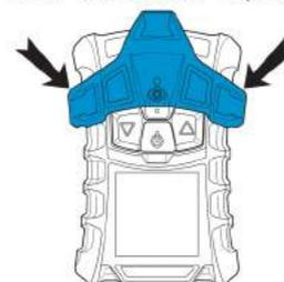
Press the ON/OFF button to start the bump test then open the valve on the regulator. The hour-glass will flash and the sensors will respond to the gas.
