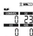
After the Bump Test completes, the device momentarily displays "BUMP PASS" or "BUMP ERROR" along with the label of any sensor that failed before returning to Measure mode. If the device fails the Bump Test, return unit to HSS Hire.
