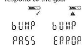
The "tick" symbol will be displayed in the Measure mode for 24 hours after a successful Bump Test.
