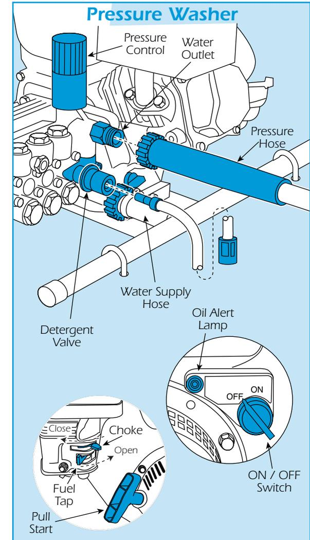
Check the engine oil and fuel levels, (see EQUIPMENT CARE').
