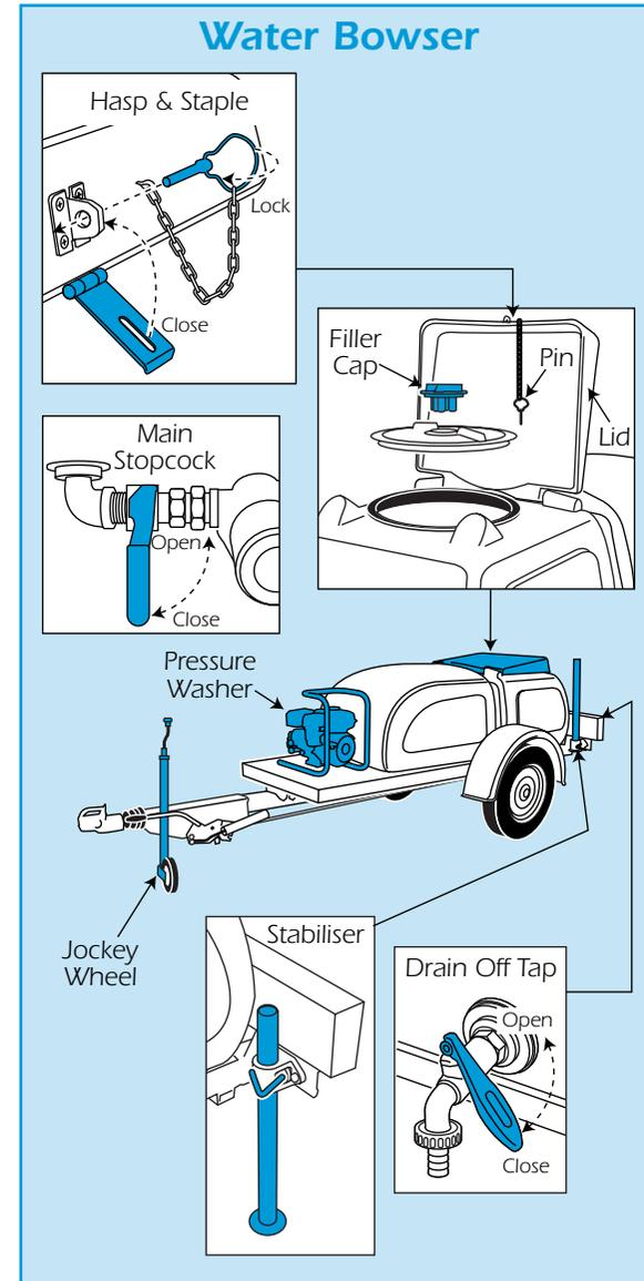
Fill the bowser until the water is no more than 300mm from the top, then turn off the supply and close and lock the filler cap.
