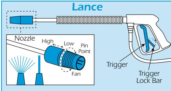
**The spray pressure can be adjusted at the spray lance.** For low pressure slide the nozzle forward and for high pressure slide the nozzle back.
