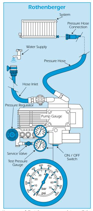
You can now Adjust the pressure regulator until the PUMP GAUGE reads the required test pressure. Turn this clockwise to increase the pressure, anti clockwise to decrease it.
