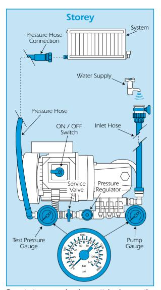
Once test pressure has been attained, open the service valve, wait unit both pump and test pressure gauges give identical readings then close the service valve and switch the pump OFF.
