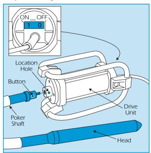
Familiarise yourself with the switches and their location so that you can operate them quickly in an emergency. Never run the unit unless it is submerged in wet concrete.
