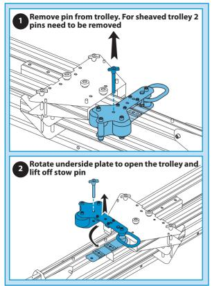
For trolleys stowed on underside upright, if stow pins available, removal can only take place when the upper A-frame assembly is rotated out of the way, or when gantry is set up.
