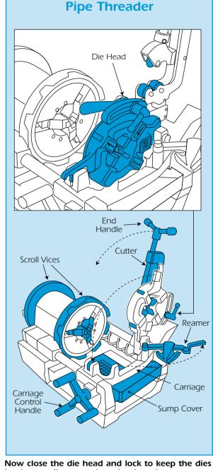
in place until mounted on the threader.
