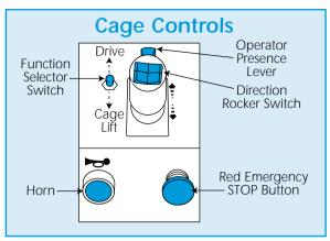
Turn the ground control selector key to the 'cage' position and check that the red emergency STOP button is pulled out to the ON position.
