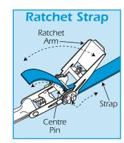
To secure the straps, open the ratchet arm. insert the loose end strap through the slot in the centre pin and pull through any excess.
