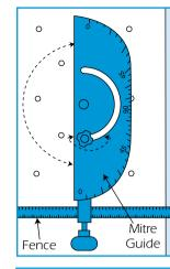
For normal straight cuts, rest the tile against the fence. Where the same cut has to be made in several tiles, set the guide at 90° to the fence and lock in position as required.
