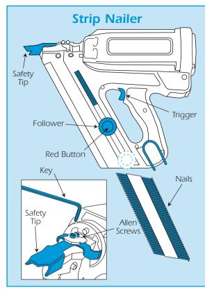
facing forward (see illustration). **Press the spring** release lever and the follower will automatically spring up and hold the strip in position.
