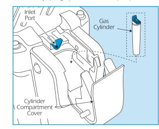
Take a gas cylinder and remove it's top protective cover and refit the dosage valve to the cylinder. Open the cylinder compartment cover on the tool (see illustration) and make sure the colour on the dosage valve corresponds with the colour of the inlet port. **Insert the cylinder**, aligning the dosage valve outlet tube with the inlet port and close the compartment cover.
